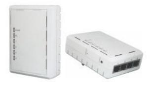
The SGN114 HomePlug AV 4-Port Ethernet Bridge operates on the HomePlug Powerline AV Specification standard, providing up to 200Mbps bandwidth over home AC wiring. Combined with a broadband DSL/Cable connection, every room
